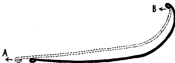
Fig. 2.—Side attachment to arch wire made of .040 steel wire, solid line showing passive position. Dotted line shows position of wire after rubber is attached at A. Distal recoil pressure exerted at B.
