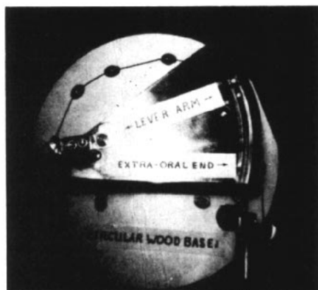
Fig. VI-1 Plan view of force-deformation instrument for testing cheek extensibility.
