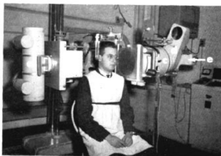
Fig. 1 Cinefluorographic unit: a. rotating anode x-ray tube, b. Videx cone adaptor, c. image intensifier, d. binocular mirror system, e. auricon camera, f. headpositioner.
