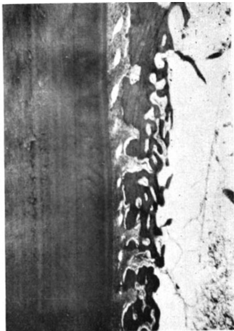
Fig. 5A Photomicrograph (x40) showing that the reaction extends the full length of the root.
