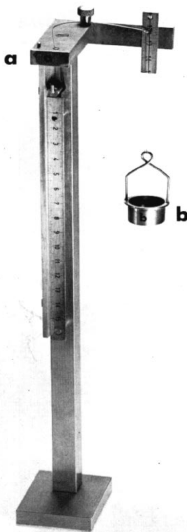
Fig. 4 Apparatus for determining the elastic and plastic deformation of a straight segment of a standard archwire. The wire is placed on the platform a so that the free loop lies on the perpendicular line on the smaller scale. The load b displaces this loop along the scale, the magnitude of the deformation being read off directly.
