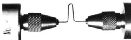
Fig. 2 Wire loop positioned in fixture in testing instrument.
