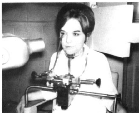
Fig. 2 Subject seated in the Panorex dental x-ray machine, her head oriented with the new cephalostat.
