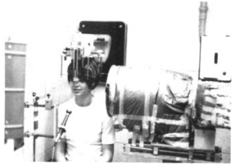
Fig. 2 Subject positioned in the modified cephalostat prior to cineradiographic registration. The intensifying screen and high speed camera are to the right.
