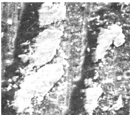
Fig. 13 Etched enamel-polished resin interface. Remaining resin removed with steel bur prior to polishing (x 700).
