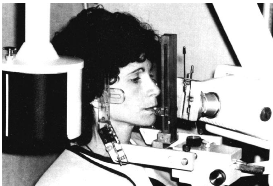
Fig. 6 Panoramic head positioner — the head is oriented and stabilized by the two earrods and incisor guide. Collimator pointer rods are retracted, ready for the x-ray exposure.
