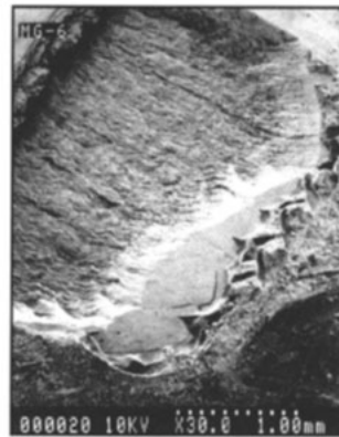
Figure 8B SEM showing the enamel surface following debonding of the metal bracket. Note defect in the enamel surface that occurred as a result of enamel fracture (x 30)
