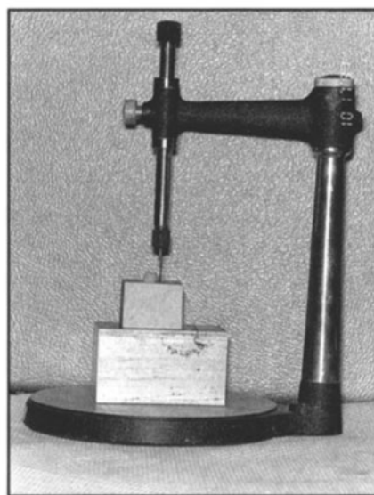
Figure 1 Dental surveyor used to orient brackets when teeth were mounted
