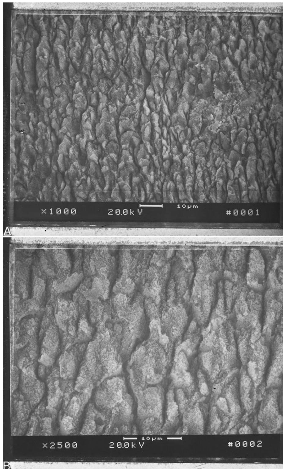
FIGURE 1. Scanning electron microscope photographs of surface enamel etched with 37% phosphoric acid at (a) 1000 \times and (b) 2500 \times . Notice the roughness of the etched enamel surface that provides significant mechanical retention during the bonding process.
