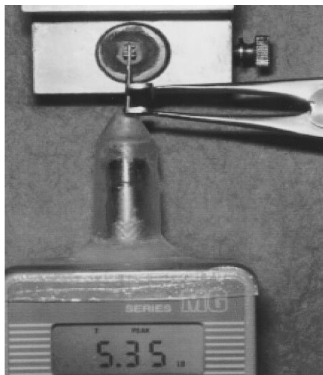
FIGURE 4. In vitro debonding using the debonding device.
