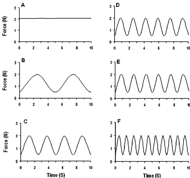
**FIGURE 3.** Waveforms of static force (A) and sine-wave cyclic forces (B)–(F) at 2 N applied to the maxillary incisors. In (B) through (F), forces were preprogrammed to oscillate from 0.2 Hz (B) to 1 Hz (F) in 0.2 Hz increments. Despite the same 2-N peak magnitude, static force lacked appreciable oscillation in force magnitude.
