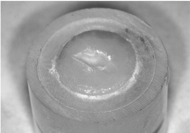
FIGURE 1. Surface destruction categorized as fracture, indicating obvious defect on porcelain surface.
