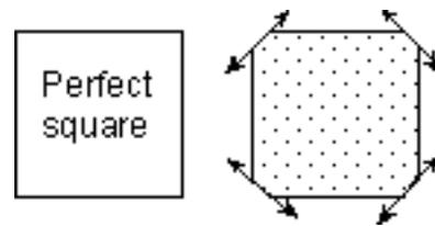
FIGURE 5. Section view of a "blunt" square wire.
