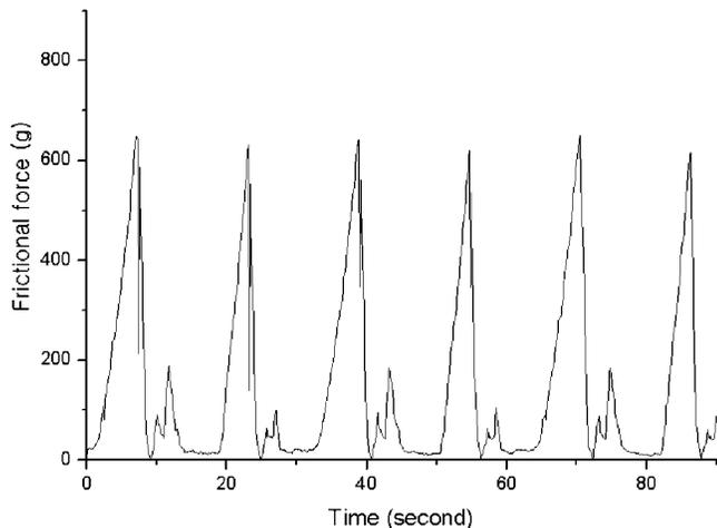
**FIGURE 3.** Time-frictional force curve for ORM-SS2 couple (ORM indicates Ormco; SS2, stainless steel 2).
