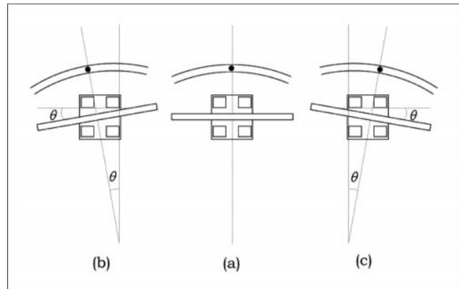
FIGURE 2. The motion of gradual change of angle between a bracket and an archwire by the pin on type friction tester.
