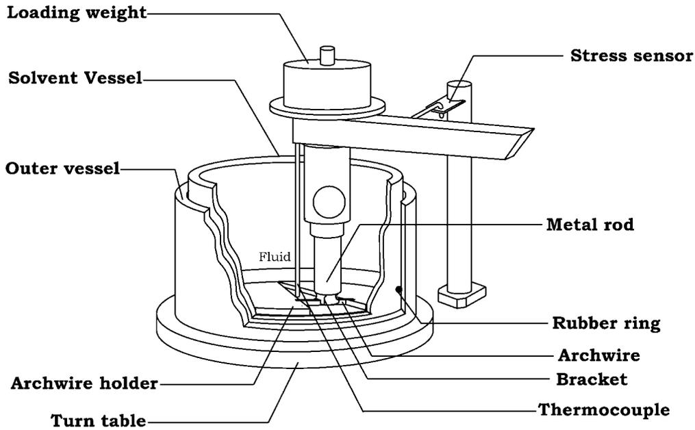
FIGURE 1. The pin on disk type friction tester used in this study.
