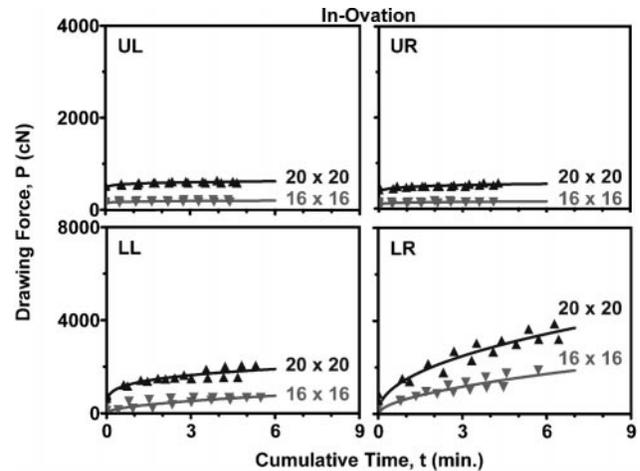
**FIGURE 3.** For the In-Ovation brackets of experiment 1, influence of the P values against t as detailed in Figure 1 using two sizes of the three manufacturer-suggested AWs: 16  $\times$  16 mils (0.016  $\times$  0.016 inch) NiTi SE and 20  $\times$  20 mils (0.020  $\times$  0.020 inch) NiTi SE.
