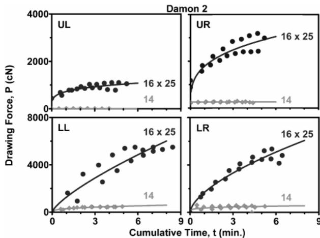
**FIGURE 4.** For the Damon 2 brackets of experiment 1, influence of the P values against t as detailed in Figure 1 using two sizes of the three manufacturer-suggested AWs: 14 mils (0.014 inch) NiTi SE and 16 × 25 mils (0.016 × 0.025 inch) NiTi SE.
