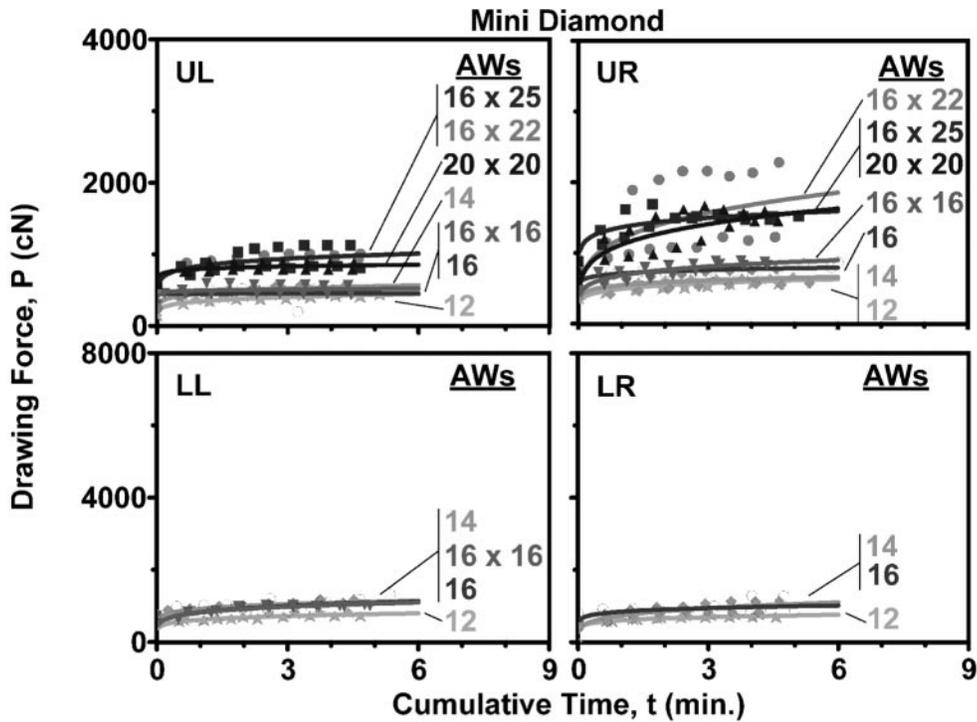
**FIGURE 5.** For the Mini Diamond brackets (control) of experiment 2, variability of the P values against t for the seven AWs (mils) tested (see shaded regions of Table 1 for AW material information). Graph displays the regression curves and data points for each AW tested.
