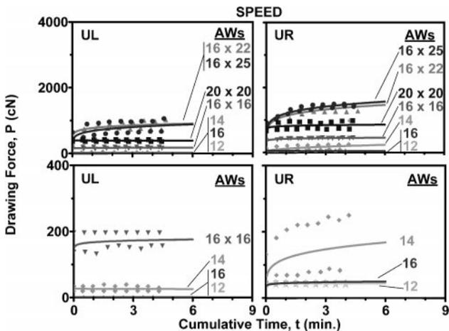
**FIGURE 6.** For the SPEED brackets of experiment 2, variability of the P values against t in two quadrants for the seven AWs (mils) tested (see shaded regions of Table 1 for AW material information). The lower frames amplify the upper frames that had P values less than 400 cN. For each AW size tested, the graph displays the combined regression of two samples. Data points not seen here were reported in a previous figure corresponding to SPEED brackets (Figure 1).
