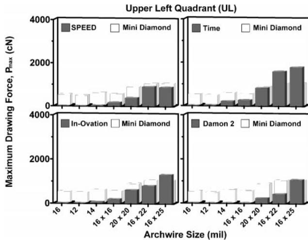
**FIGURE 10.** For the UL quadrant of experiment 2, the maximum drawing force ( $P_{max}$ ) values for all seven AW sizes tested. The graph compares the  $P_{max}$  values of the self-ligating designs (□) with the  $P_{max}$  values of the conventional (■) design.
