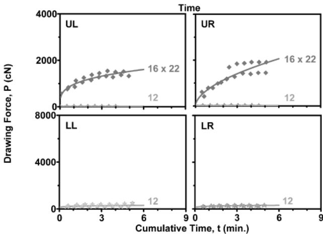
**FIGURE 2.** For the Time brackets of experiment 1, influence of the P values against t as detailed in Figure 1 using two sizes of the three manufacturer-suggested AWs: 12 mils (0.012 inch) NiTi and 16  $\times$  22 mil (0.016  $\times$  0.022 inch) NiTi.
