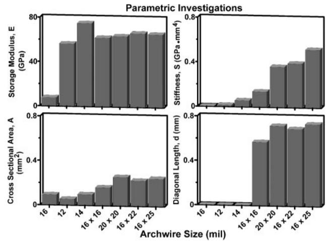
**FIGURE 12.** Bar graphs of four parameters (storage modulus [E], bending stiffness [ $S = I \cdot E$ ], cross-sectional area [A], and diagonal length [d]) calculated by dimensional measurements or thermal analyses for the seven AW sizes tested. For experiment 2, the best correlation occurred when  $S = I \cdot E$ .
