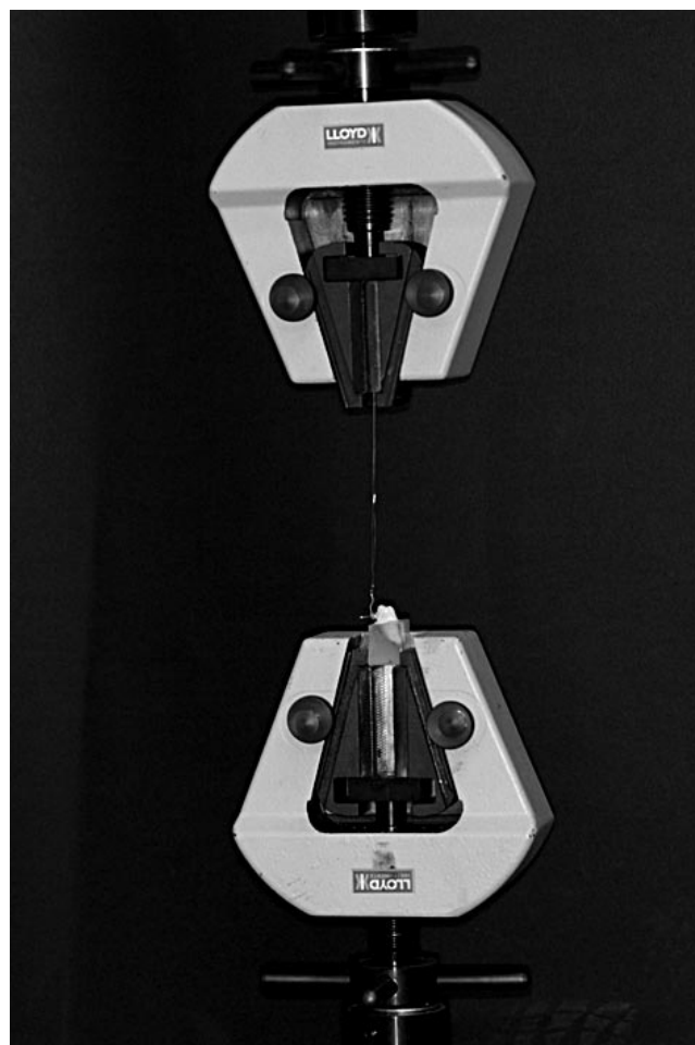
FIGURE 2. Bonded teeth set in acrylic block and positioned in a testing machine.
