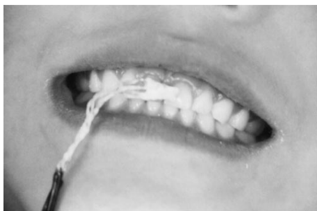
FIGURE 4. Transducer used in the labial surface of the upper incisor.
