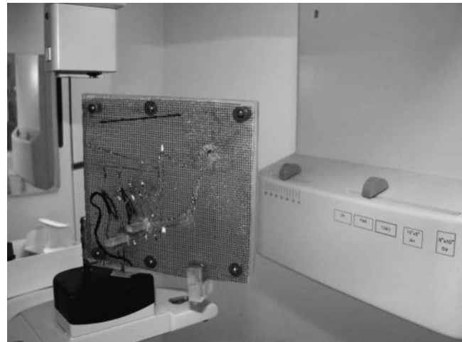
FIGURE 1. The phantom was set up in the panoramic machine using a custom positioner that was representative of an average mandibular position in the machine.
