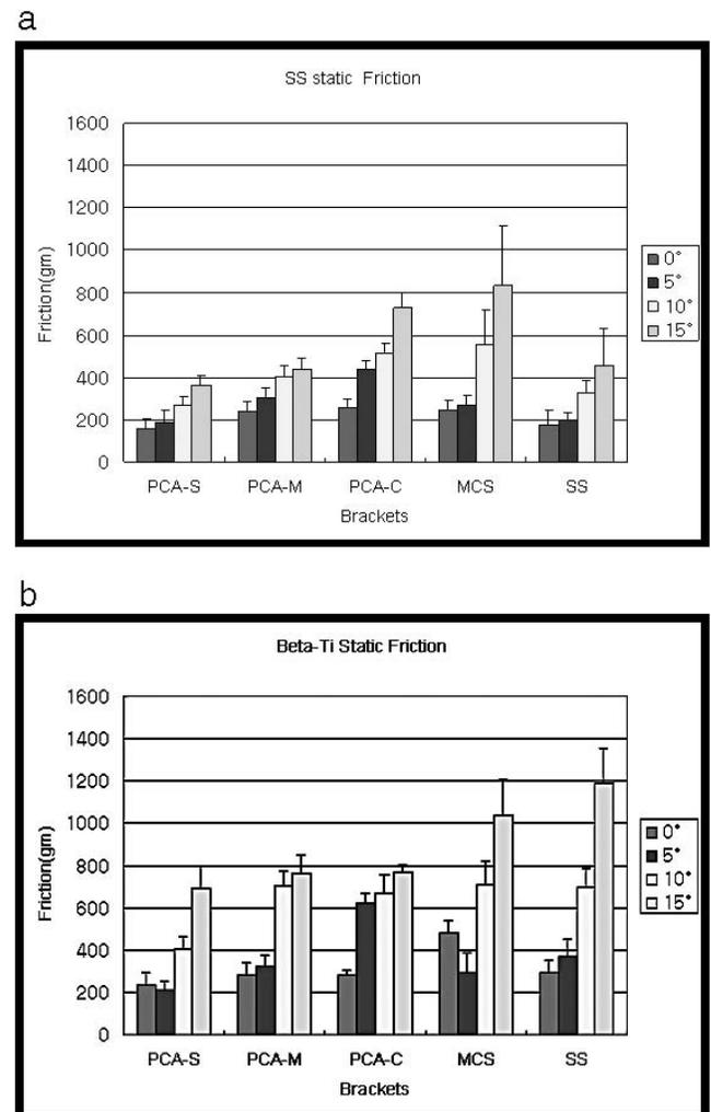
**Figure 4.** Static mean friction between at the four angles (0°, 5°, 10° and 15°). Note graph showing the increase in friction with increased tipping angle. (A) Static mean friction between SS wire/bracket combinations. (B) Static mean friction between  $\beta$ -Ti wire/bracket combinations.
