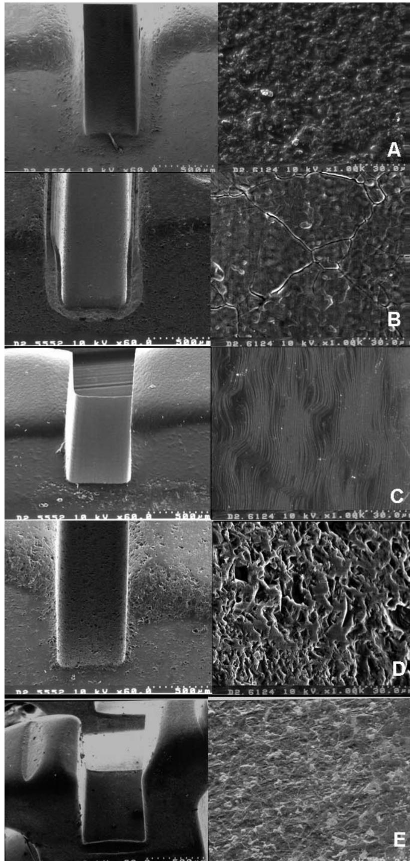
**Figure 5.** Scanning electron micrographs of brackets at 60× and 1000× magnification. (A) PCA-S; (B) PCA-M; (C) MCS; (D) PCA-C; (E) SS.
