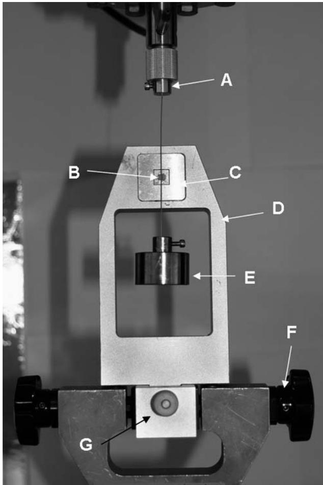
**Figure 2.** Testing machine, bracket-wire assembly, and force measuring equipment. (a) Rotation fixture. (b) Inner aluminum block. (c) Outer aluminum block. (d) Anterior-posterior adjustable block. (e) Weight (150 g). (f) Horizontal adjustable joint. (g) Anterior-posterior adjusting handle.
