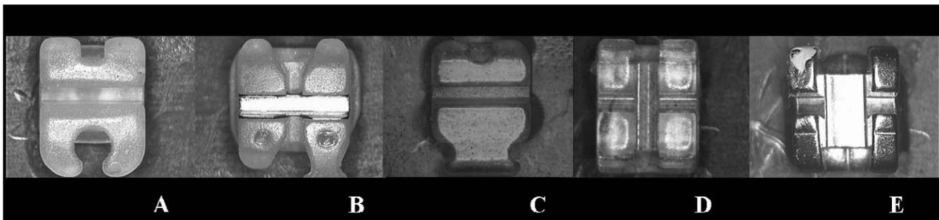
**Figure 1.** Tested brackets: (A) PCA-S; (B) PCA-M; (C) PCA-C; (D) MCS; (E) SS (magnification 20×).
