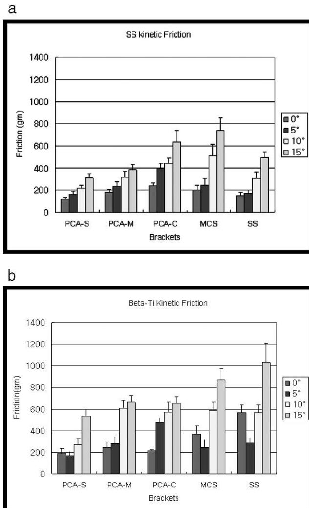
**Figure 3.** Kinetic mean friction between the four angles (0°, 5°, 10°, and 15°). Note graph showing the increase in friction with increased tipping angle. (A) Kinetic mean friction between SS wire/bracket combinations (B) Kinetic mean friction between  $\beta$ -Ti wire/bracket combinations.
