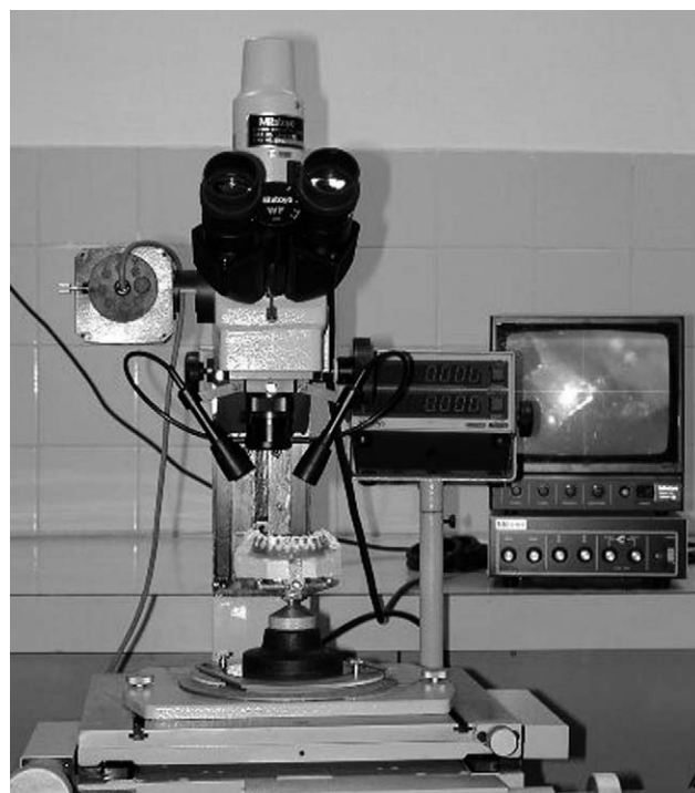
Figure 2. A setup model is placed in a toolmaker's microscope for measuring RotD in millimeters.
