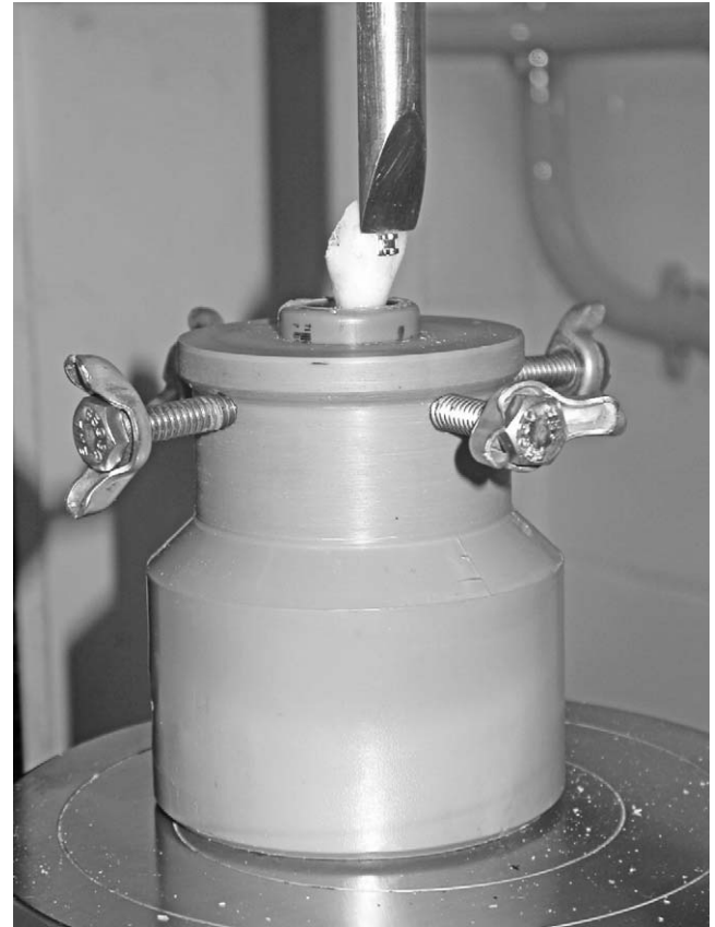
Figure 1. View of the bond strength test setup.
