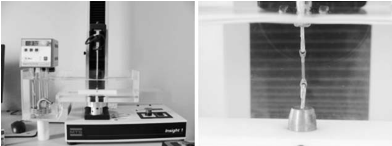
Figure 3. Force application device with load cell and computer calibration.
