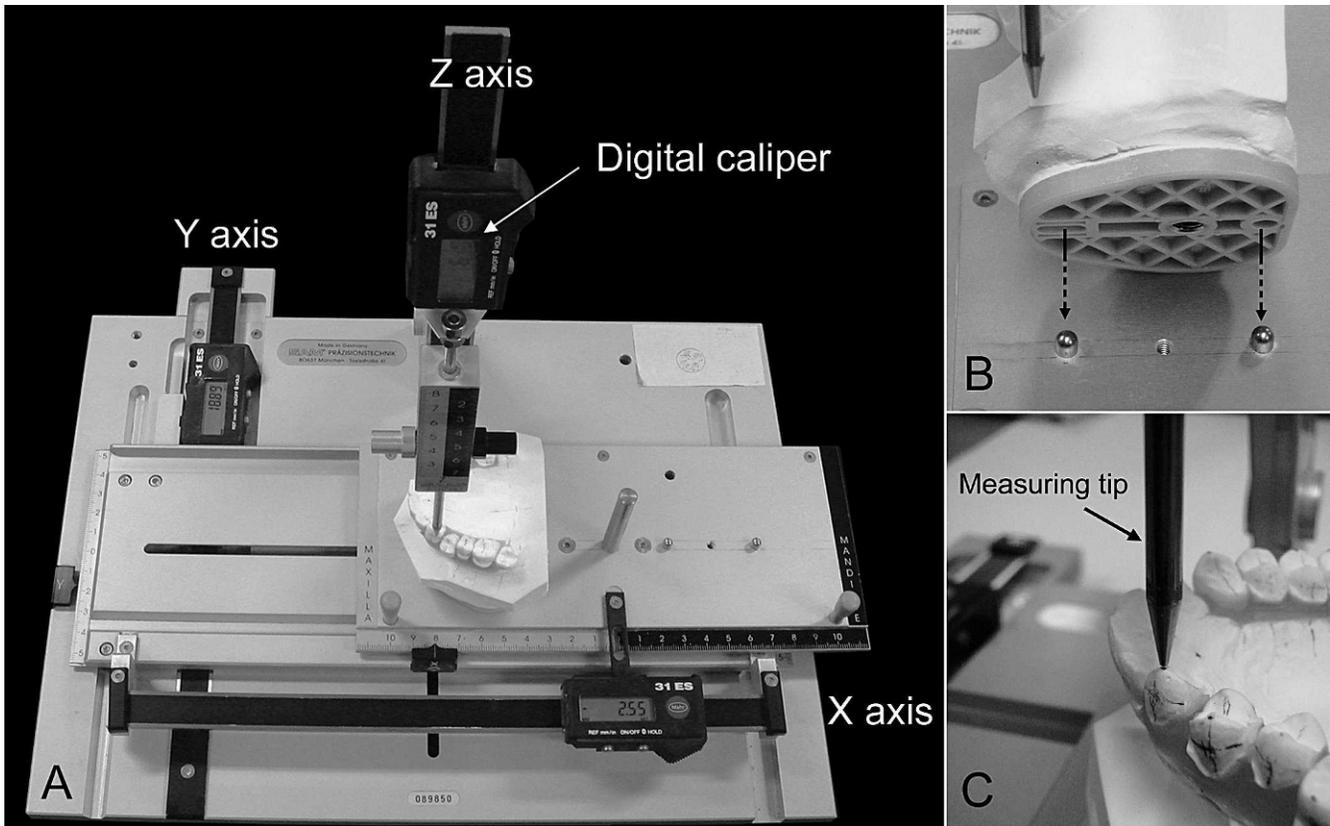
**Figure 2.** Measurement of the plaster model with the Reference Measurement Instrument (RMI). (A) Digital calipers in the x-, y-, and z-axes. (B) Plaster model, which could be placed repeatedly in the same position on the RMI. (C) Measuring tip on the canine.
