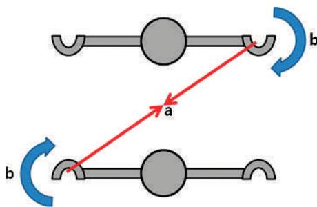
**Figure 2.** A schematic diagram of clockwise loading on lever-arm-shaped upper structures. a indicates the direction of force; b, clockwise moment.
