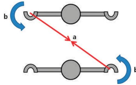
**Figure 3.** A schematic diagram of counterclockwise loading on lever-arm-shaped upper structures. a indicates the direction of force; b, counterclockwise moment.
