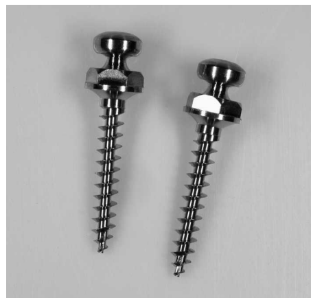
Figure 1. Two microimplants with mushroom head for comfort (1.6 mm diameter, 10 mm length).
