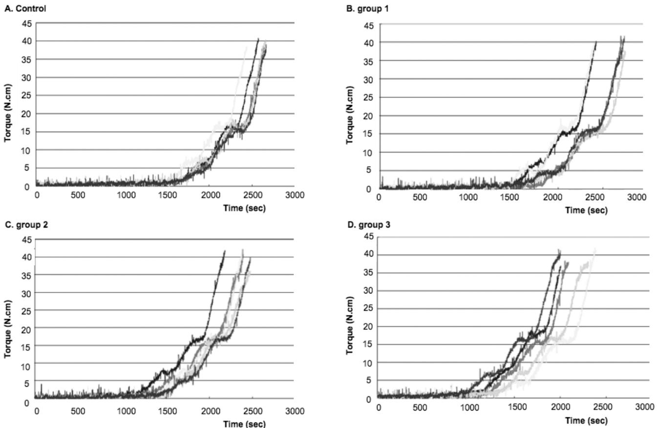
**Figure 2.** Graph of insertion time and torque during the insertion of five different samples in the control group (A), group 1 (B), group 2 (C), and group 3 (D). The overall changes in torque were similar among different groups; however, insertion time (arrow) varied according to the loading condition.
