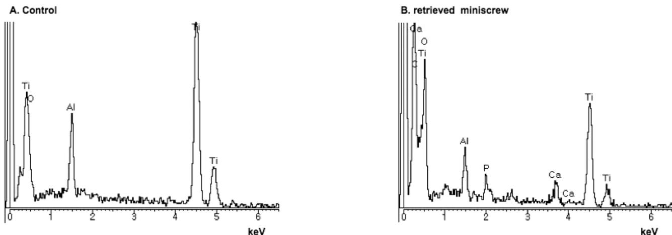
**Figure 3.** Elemental analysis of the miniscrew surface. (A) Titanium (Ti), oxygen (O), and aluminum (Al) were evident on the control miniscrew surface. (B) Foreign elements such as carbon (C), calcium (Ca), and phosphorus (P) were additionally evident on the retrieved miniscrew surface.
