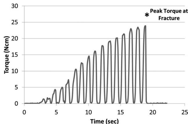
**Figure 3.** A representative graph of insertion torque against time for the Aarhus mini-implant. The asterisk (\*) represents the maximum insertion torque just prior to mini-implant fracture.
