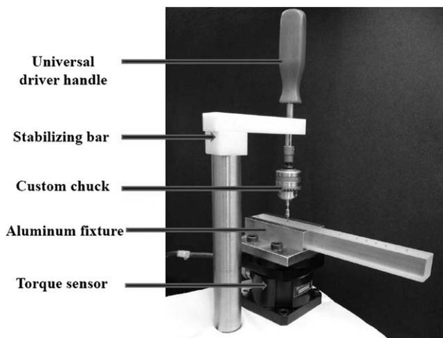
**Figure 2.** Experimental apparatus used for fracture testing.
