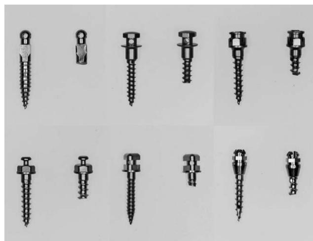
**Figure 5.** Fracture position of the mini-implants tested. Upper row from left to right: Unitek, Aarhus, OrthoEasy. Lower row, from left to right: Dual-Top, VectorTAS, Tomas-pin. All fractured within the threaded portion of the mini-implant body.
