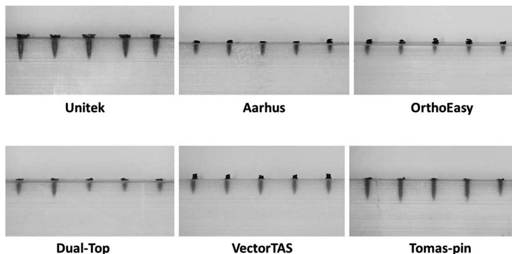
**Figure 6.** Photographs showing the level of mini-implant fracture. All mini-implants failed at the level of the acrylic block, leaving up to 1 mm of mini-implant exposed.
