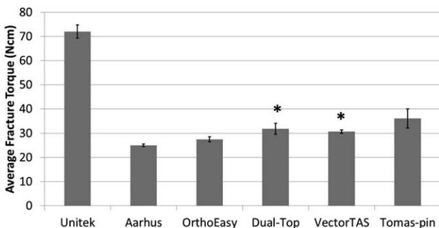
**Figure 4.** Bar graph showing the mean fracture torques for various mini-implant manufacturers (mean ± SD; n = 15). All differences were significant ( $P < .05$ ), except the difference between Dual-Top and VectorTAS ( $P = .744$ ), indicated by the asterisk (\*).
