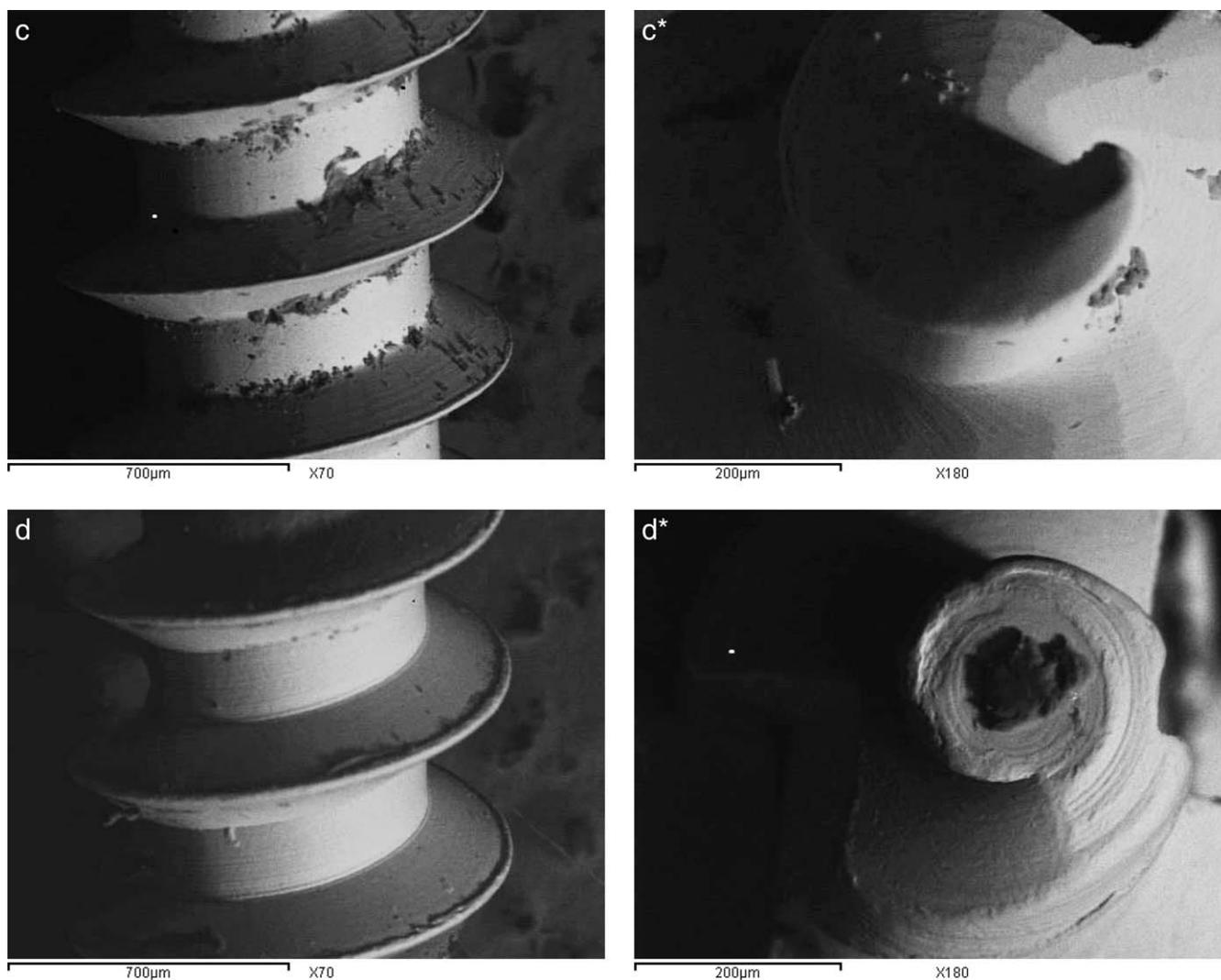
**Figure 2.** (c) SEM at magnification  $\times 70$  showing the flutes of a retrieved micro-implant sterilized by gamma radiation. (c\*) SEM at magnification  $\times 180$  showing the tip of the same micro-implant. (d) SEM at magnification  $\times 70$  showing the flutes of a retrieved micro-implant sterilized by ultraviolet radiation. (d\*) SEM at magnification  $\times 180$  showing the tip of the same micro-implant. SEM indicates scanning electron microscopy.
