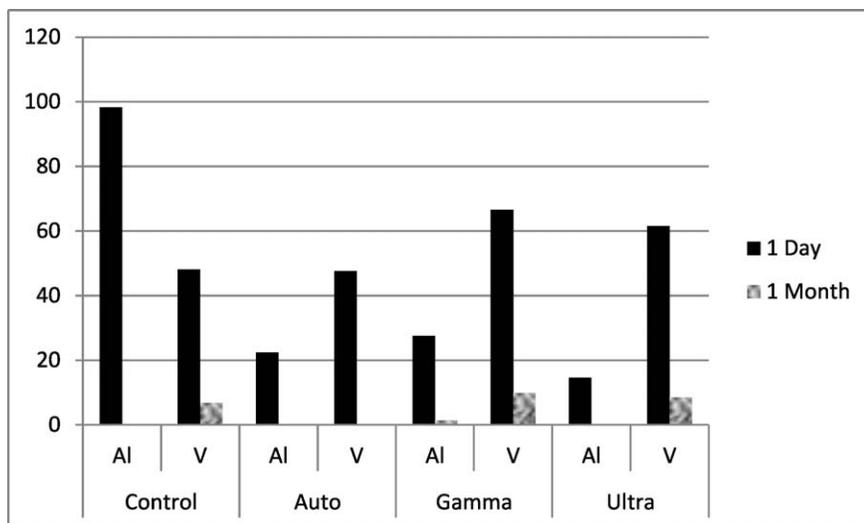
**Figure 3.** Aluminum and vanadium concentrations (in parts per billion) for the control as-received micro-implants and for the micro-implants sterilized by autoclave, gamma-rays, and ultraviolet radiation at the 1-day and 1-month immersion periods.
