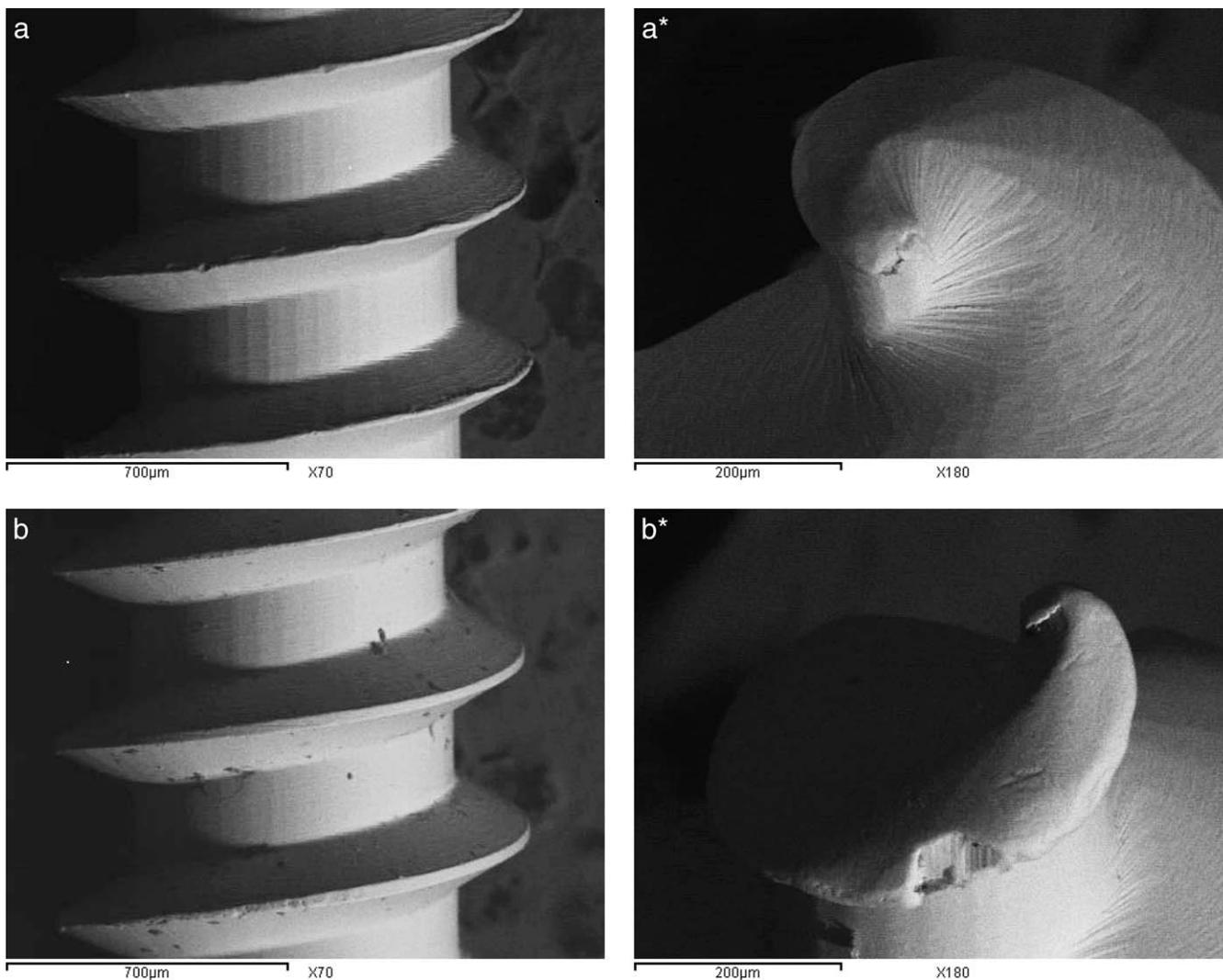
**Figure 2.** (a) SEM at magnification  $\times 70$  showing the flutes of the control as-received micro-implant. (a\*) SEM at magnification  $\times 180$  showing the tip of the same micro-implant. (b) SEM at magnification  $\times 70$  showing the flutes of a retrieved micro-implant sterilized by autoclave. (b\*) SEM at magnification  $\times 180$  showing the tip of the same micro-implant.
