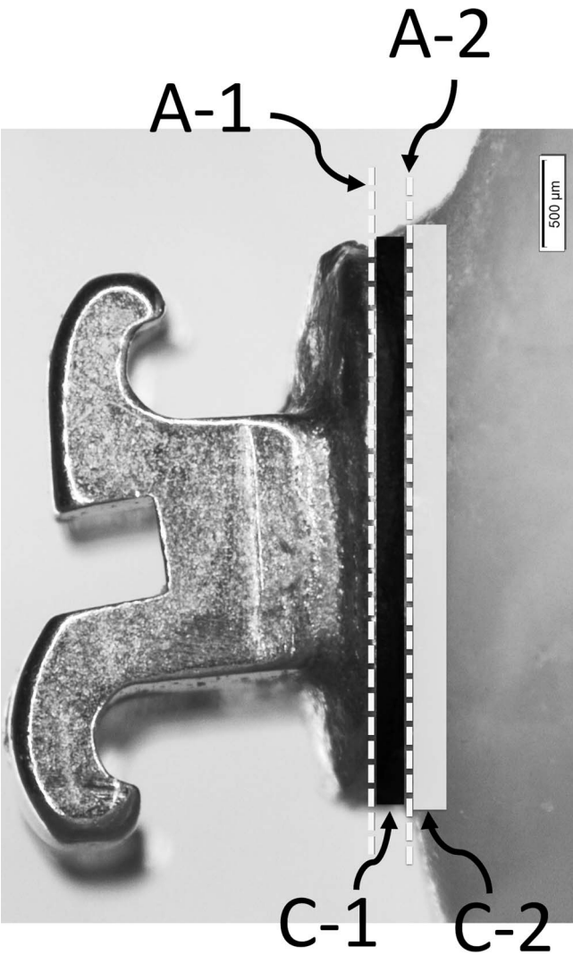
Figure 1. Diagram showing failure mode identification. Adhesive failures: Type A-1, bracket/adhesive, type A-2, adhesive/enamel. Cohesive failures: type C-1, within the adhesive layer; type C-2, within enamel. Mixed mode failures: a combination of adhesive and cohesive failures.
