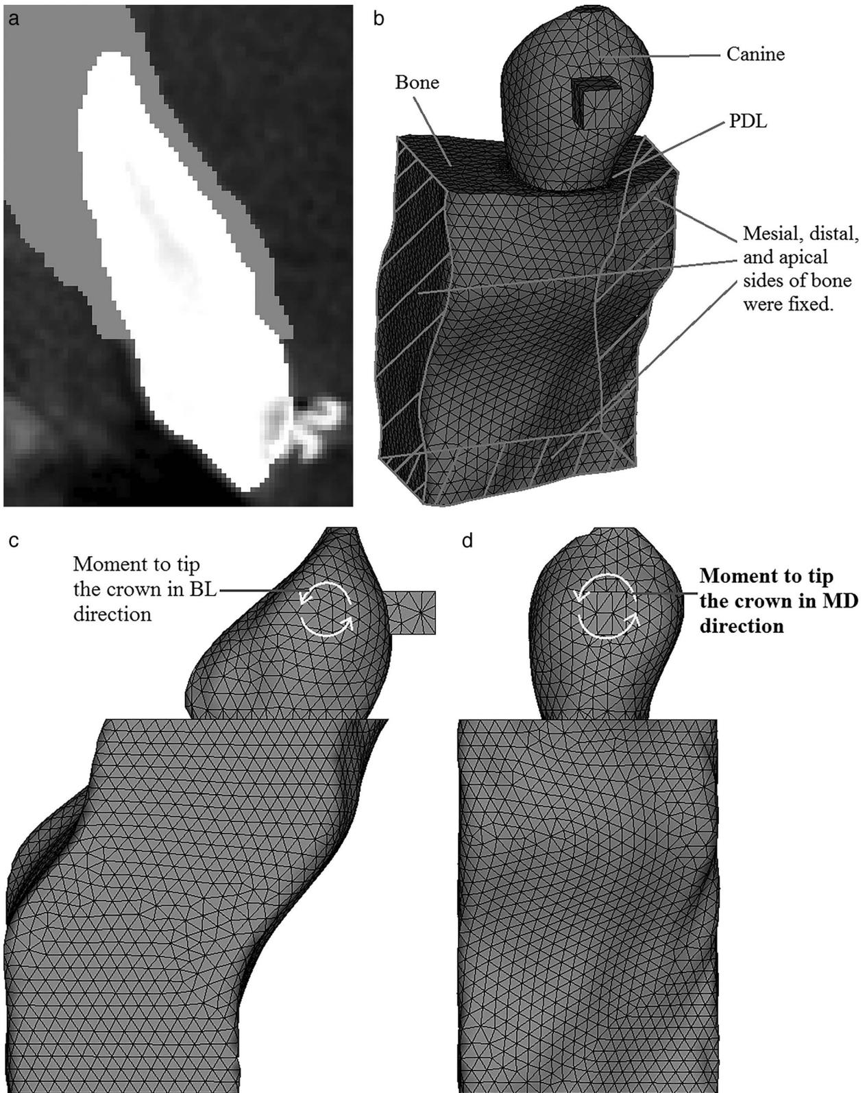
**Figure 1.** Creation of the finite element models. (a) Segmentation of the root and bone. (b) Meshes and boundary conditions. (c) Loading condition in the BL direction. (d) Loading condition in the MD direction.
