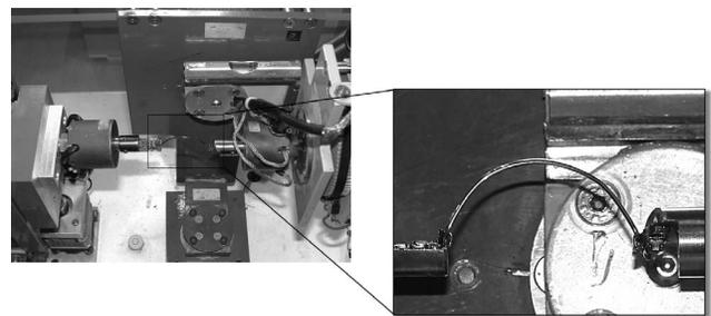
**Figure 2.** The force system identification testing machine showing the two sensors attached to lingual tubes in which the terminal ends of the transpalatal arches were inserted.
