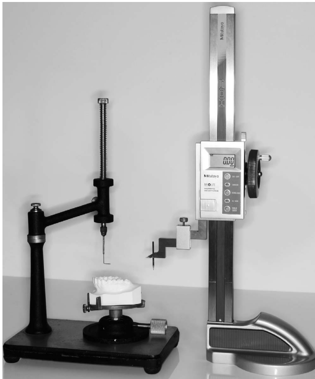
Figure 1. Instruments used in this study. Standardization of the dental cast position was obtained using an L-shaped accessory attached to a parallelometer. Tooth measurements were performed with a digital height gauge with 0.01-mm precision.
