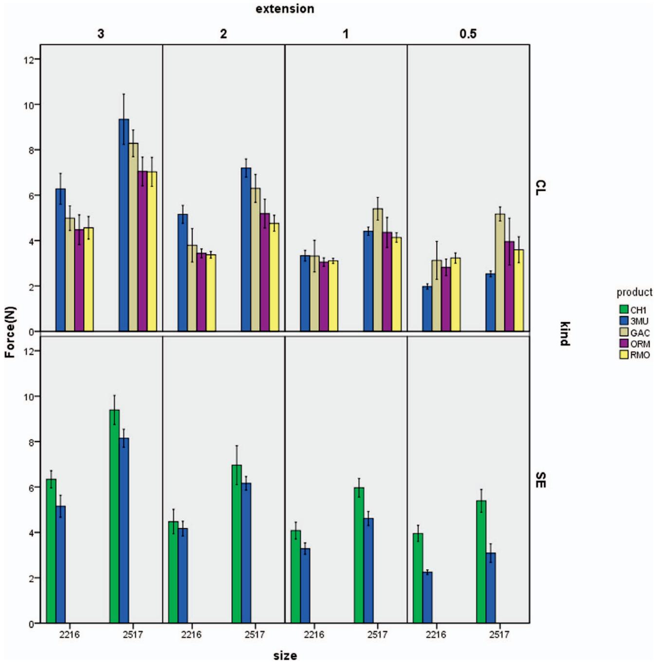
**Figure 3.** Mean deactivation force values of conventional and superelastic Ni-Ti wires at different deflections as ribbon archwires. The error bars indicate plus and minus one standard deviation from the mean.
