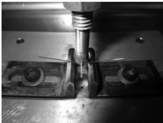
**Figure 1.** Three-point flexural test apparatus.
