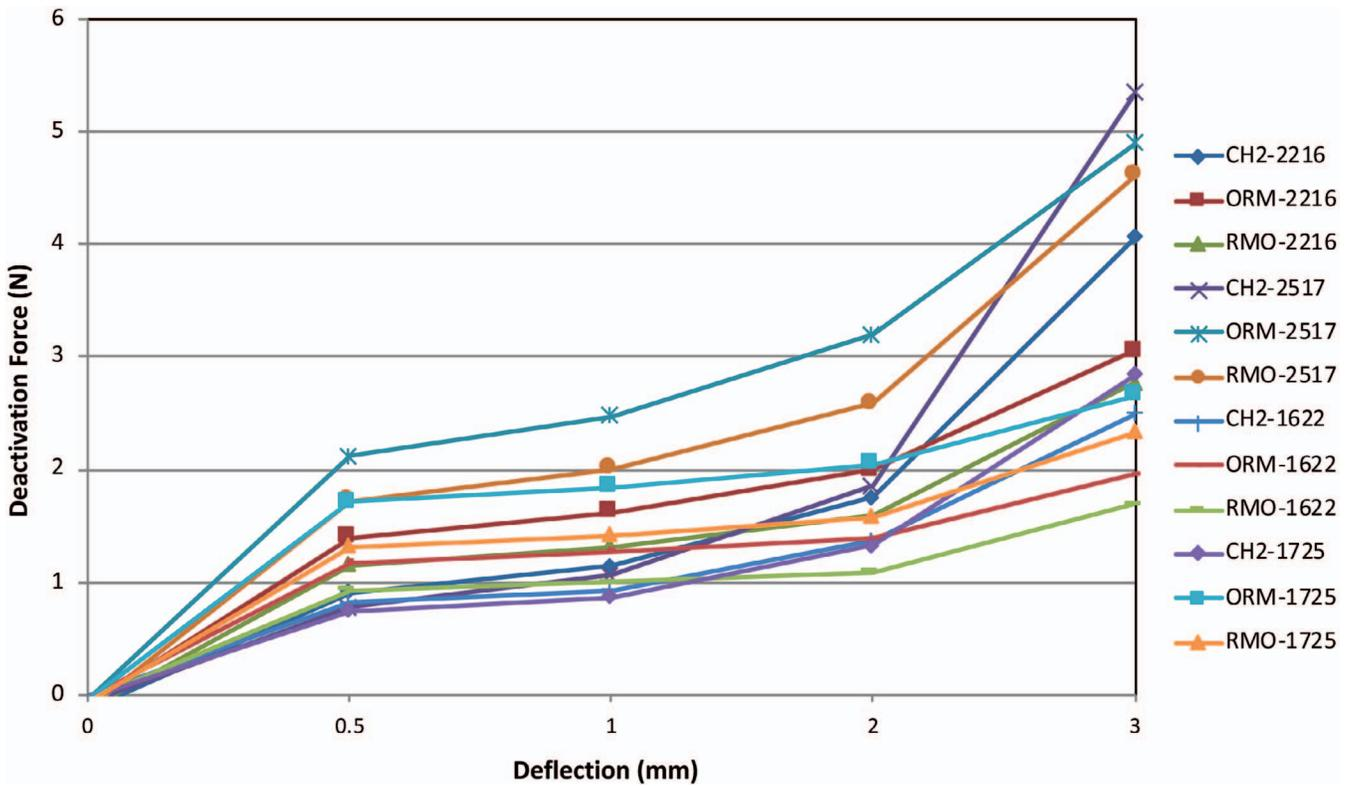
Figure 4. Mean deactivation force values of thermal Ni-Ti wires at different deflections.
