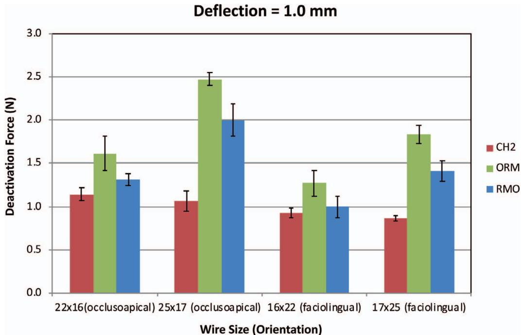
**Figure 5.** Mean deactivation force values of thermal Ni-Ti wires at 1-mm deflection. The error bars indicate plus and minus one standard deviation from the mean.
