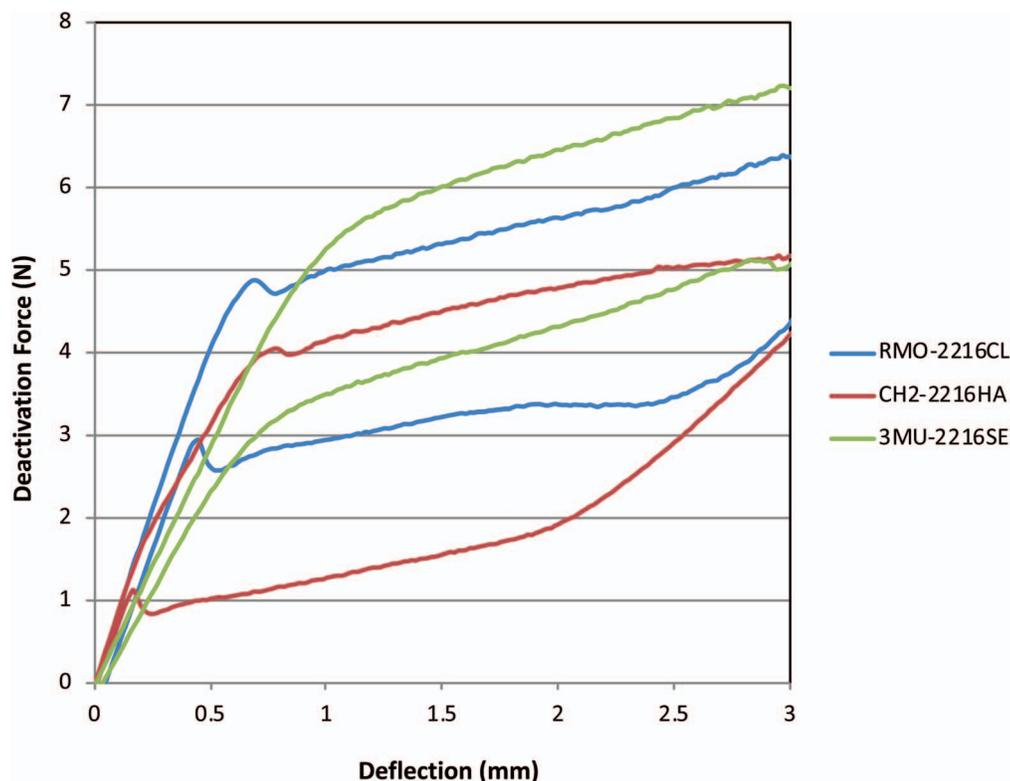
**Figure 2.** Representative force-deflection plots of three kinds of Ni-Ti archwires in occlusoapical orientation.
