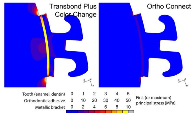
**Figure 4.** Shrinkage stress distributions of the first (maximum) principal stress generated by polymerization of two orthodontic adhesives that represented the highest and lowest shrinkage stress levels of the six materials evaluated.
