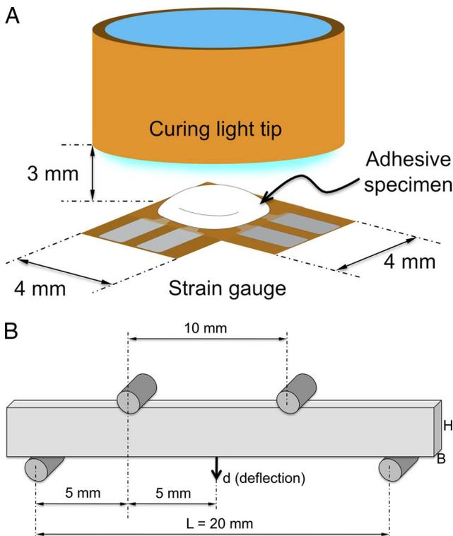
**Figure 1.** (A) Adhesive specimen placed on biaxial strain gauge and cured from the top. (B) Four-point bending bar configuration and dimensions.
