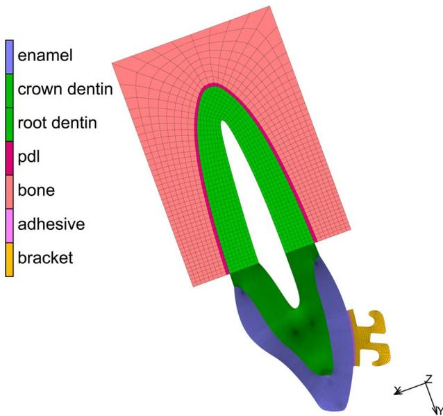
**Figure 2.** Cross-sectional finite element model of incisor with stainless steel bracket.
