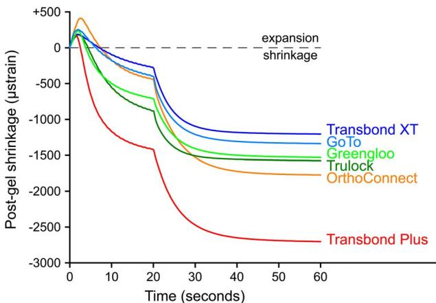
**Figure 3.** Mean strain curve for each of the six orthodontic adhesives during the first 60 seconds after start of polymerization, showing initial expansion (positive strains) followed by shrinkage (negative strains).
