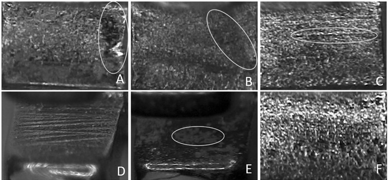
**Figure 3.** Morphological features (circled) visible on OLM images of used brackets (A–E) (mag. 60×) and on new brackets (F); (A) wear/abfraction, (B) discoloration, (C) pits/crevices, (D) striations, (E) adherent material, (F) bottom.
