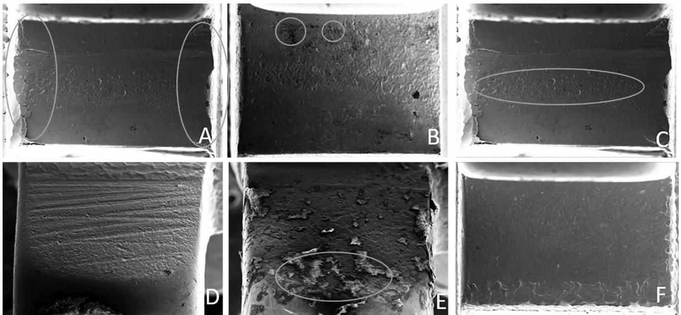
**Figure 4.** Morphological features (circled) visible on SEM images (300× magnified) of used brackets (A–E) and on new brackets (F); (A) wear/abfraction, (B) discoloration, (C) pits/crevices, (D) striations, (E) adherent material, (F) bottom.
