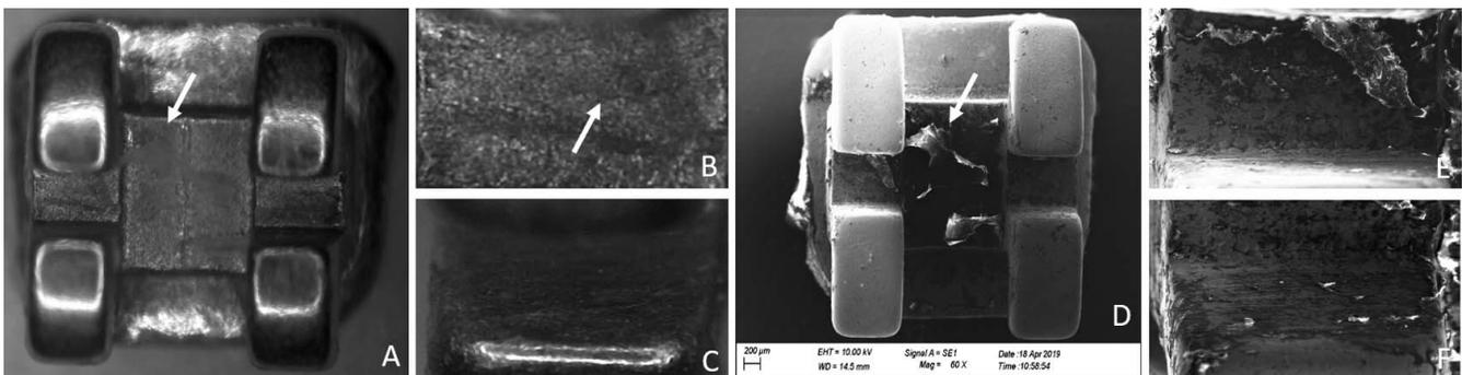
**Figure 6.** OLM (A–C) and SEM (D–F) images (image D 60 $\times$ , images E&F 300 $\times$  magnified, used bracket) (A, D) adhesive material visible in the middle bracket area (white arrow); (B, E) the bottoms of the bracket slots with visible red-brown discoloration (white arrow), wear, and deformation of the external edges; (C, F) cervical walls.
