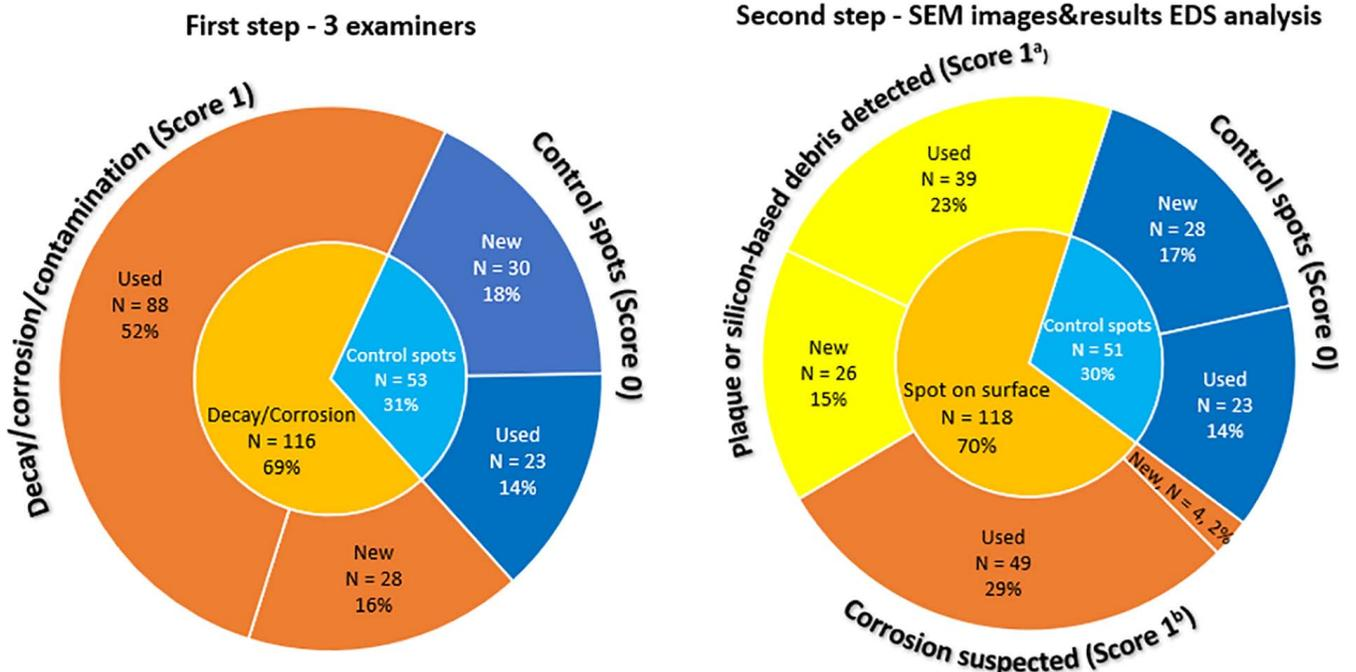
**Figure 7.** Qualitative surface assessment discriminating between control spots, contaminated spots, and corrosion-suspected spots.
