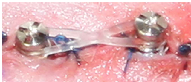
Figure 2. Miniscrews in rabbit tibia with load applied.
