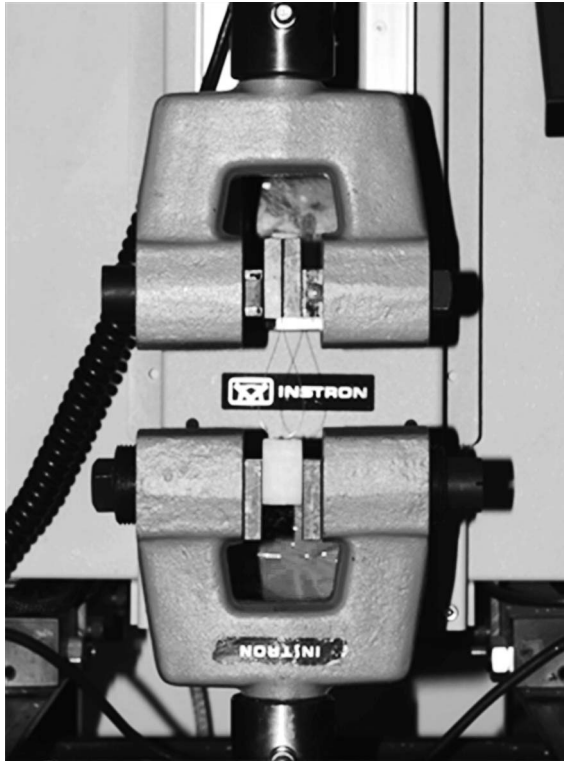
Figure 3. Experimental setup for tensile testing using an Instron machine.
