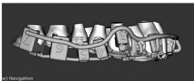
Figure 1. Computer-aided design/computer-aided manufacturing (CAD/CAM) digital tray for indirect bonding (IB).
